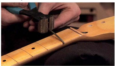
2. Once your fret has been hammered and evenly secured across the fret board, flip the neck over and apply the Hot Stuff glue to the bottom of the fret tang, on each side of the neck. The instant glue will naturally wick down inside the fret slot, fixing the fret in place.
