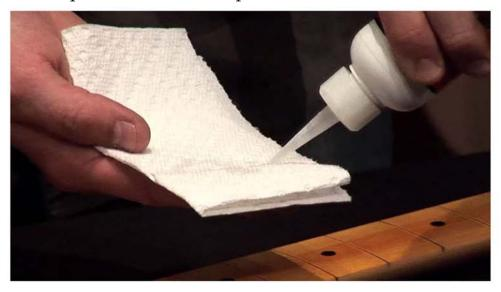
3. When applying the glue to the fret board with a paper towel, you want to move you hand in a quick, even manner across the entire surface of the board. You may want to tape off the headstock, and any other area to which you do not want to risk applying glue.
