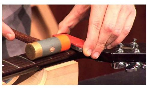
3. Using either the Super 'T' or Special 'T', gap-filling glues, evenly spread the glue across the bottom of the nut. These thicker grades of glue will fill gaps left by wood potentially removed while extracting the nut.
