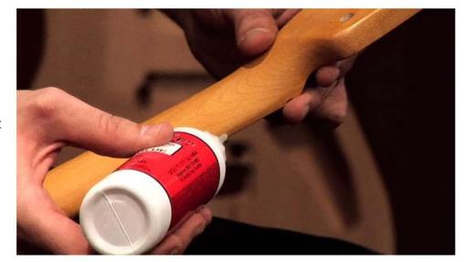
3. After you have applied the glue, turn the neck back over and spray some NCF Quick to move the process along quickly. Remember to keep the can about 12"-18" away from the surface you are spraying.
