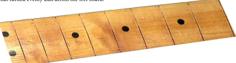
8. Once your finish has been evenly sanded, it is ready to be buffed. Depending on your method of buffing the Hot Stuff finish can be buffed to varying degrees. I light buffing job will produce a dull, satin-like finish, and extensive buffing with multiple grades of compound can produce a high-gloss, factory finish.
