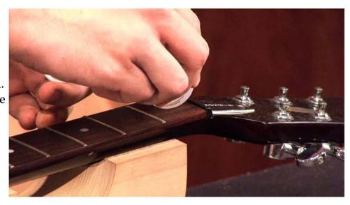
2. Using a flat piece of material (either wood or plastic), press across the whole surface of the front of the nut. This will allow the impact of the hammer to spread evenly across. Lightly tap the material until the nut loosens, or falls out of place. If the nut will not fall out of position, you can gently use end nippers to pull it up out of the slot.
